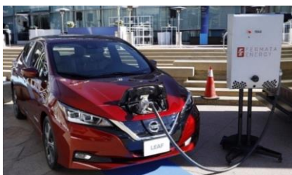
Figure 20: Nissan unveils the U.S. commercial offering of Vehicle-to-Home charging for the U.S., using battery-powered Leaf cars and Fermata Energy bi-directional charging. 51
